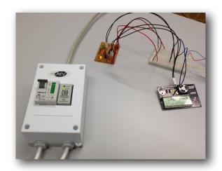
The setup shows an S0 device that measures the power consumption of the electrical equipment connected to it. We have designed a custom circuit that pulls measurements from the S0 device and sends them to the AVR Raven. The Raven converts pulses into equivalent kWh of power consumed and transfers this information via IPv6 to the collector that queries for it using SNMP.
