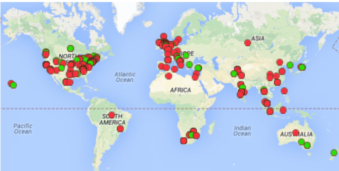
Fig. 6. The coverage of the BISmark measurement platform as of Feb 2015. The green and red dots represent connected (around 119) and disconnected probes respectively: http://networkdashboard.org .
