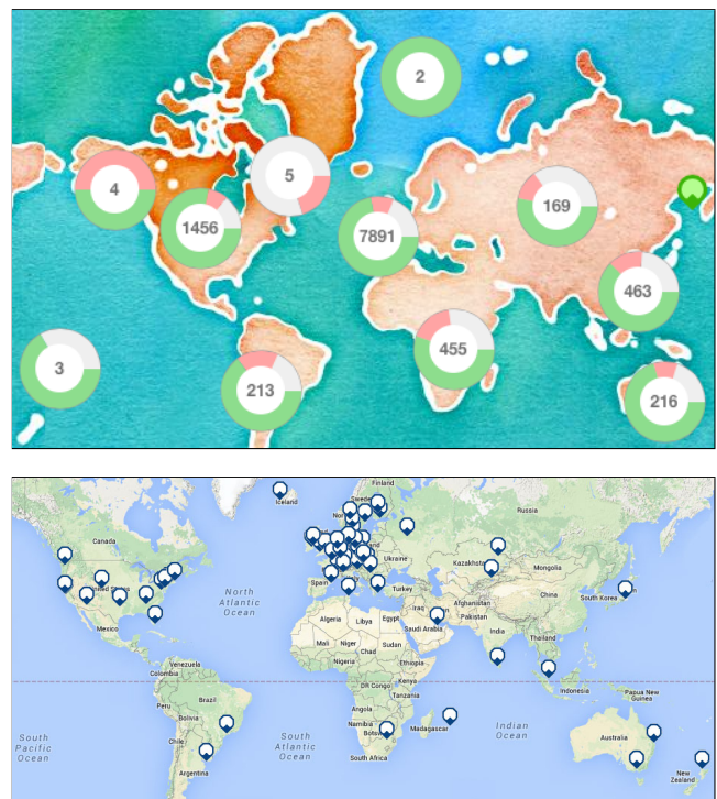
Figure 1: Coverage of the RIPE Atlas measurement platform as of Feb 2015. Around 12.8K probes (top) and 109 anchors (bottom) have been deployed in total: atlas.ripe.net/results/maps . The green, red and grey areas (above) represent connected, disconnected and abandoned probes respectively.
