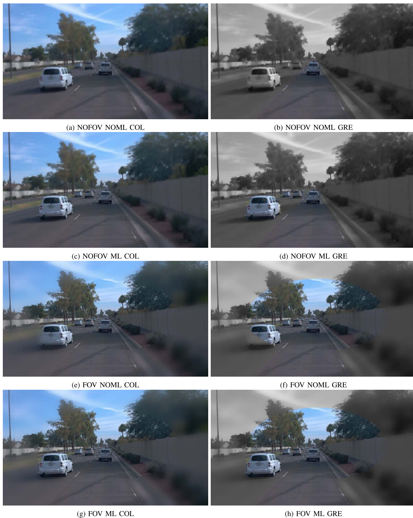
Fig. 11. Comparison of all applied approaches in the order of their introduction within the paper. Images (a)–(d) show the non FOV approach, while images (e)–(h) show the approach with applied FOV. Images (a),(b),(e),(f) show the approach without the application of ML, while images (c),(d),(g),(h) show the utilization of the ML-Eff model.
